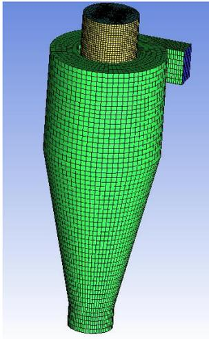
Figure 3: The hexahedral structured grid.
