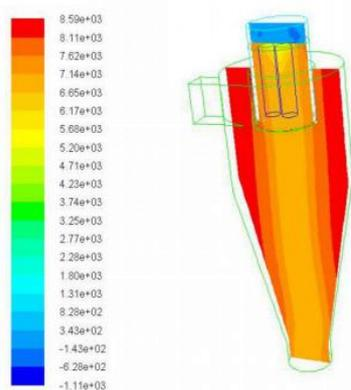
Figure 4: The pressure contour of the internal flow field.
