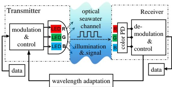
Figure 9: LED-based VLC transceiver with wavelength adaptation.
