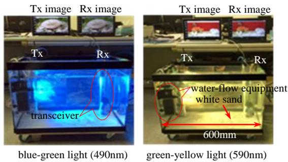
Figure 15: The results of underwater one-to-one image transmissions with different light wavelength.
