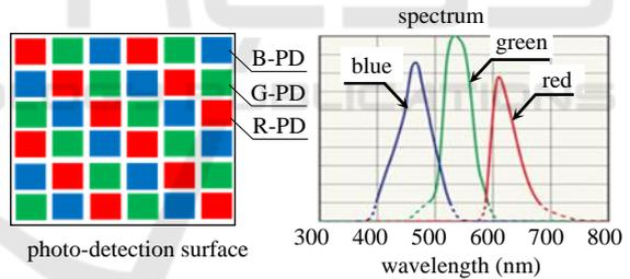
Figure 11: Three-sensors color photodiode.
