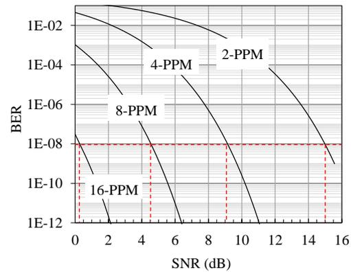
Figure 13: BER versus SNR for  $L$ -PPM with different  $L$  values.
