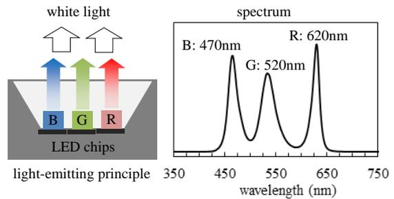
Figure 10: Three-chips white LED module.
