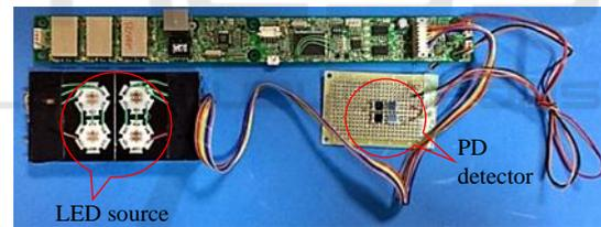
Figure 14: The prototype of LED-based VLC transceiver.
