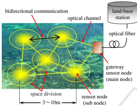
Figure 8: The mesh-type UOWSN.
