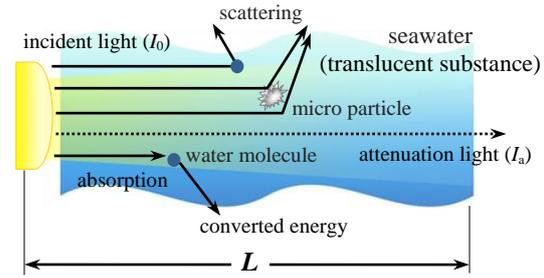
Figure 4: Physical model of light propagation in seawater.
