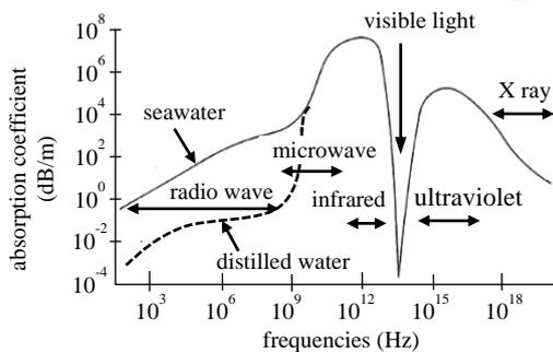
Figure 3: Absorption coefficients of electromagnetic wave in the water.
