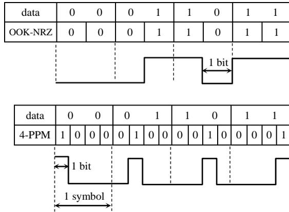
Figure 12: The coding methods of OOK-NRZ and 4-PPM.
