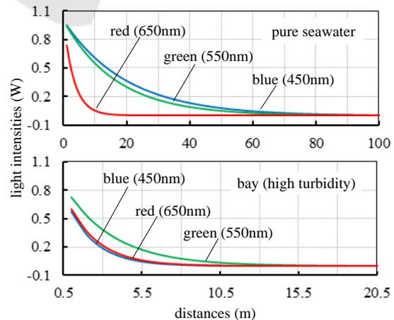
Figure 5: Spectrum-intensity attenuation for different seawater types in horizontal direction.
