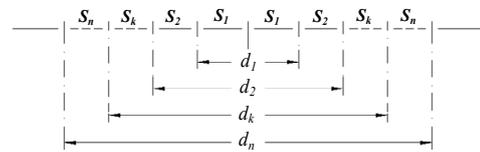
Figure 1: Multihole directional coupler.
