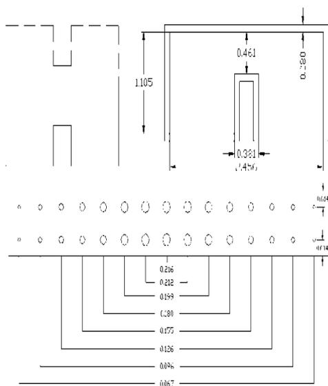
Figure 2: The structure and dimension of the directional coupler.
