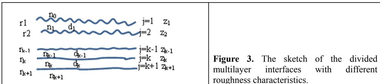
**Figure 3.** The sketch of the divided multilayer interfaces with different roughness characteristics.
