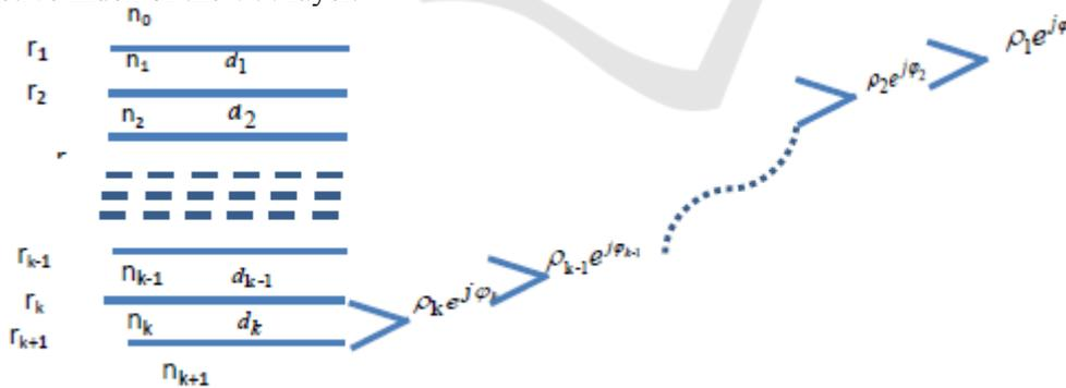
**Figure 2.** The recursive method for obtaining the Fresnel coefficient.
