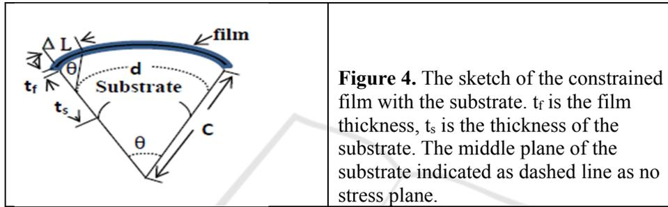
**Figure 4.** The sketch of the constrained film with the substrate.  $t_f$  is the film thickness,  $t_s$  is the thickness of the substrate. The middle plane of the substrate indicated as dashed line as no stress plane.
