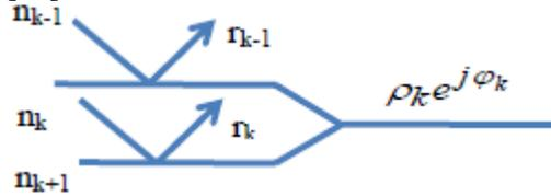
**Figure 1.** The equivalent interface of a single layer.
