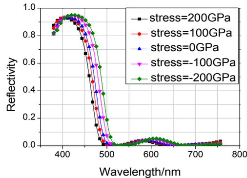
**Figure 7.** The reflectivity for different stress values with the same glass substrate thickness of 0.1 mm.
