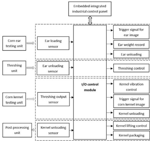
Fig.4 Overall design of control system
