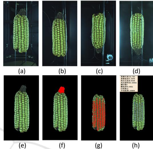
(a)Original image of Cam. 1 (b)Original image of Cam. 2 (c)Original image of Cam. 3 (d)Original image of Cam. 4 (e)Background removal for Fig.8(a) (f)bare tip extract for Fig.7(a) (g)kernel extract for Fig.7(a) (h)kernel track for Fig.7(a)
