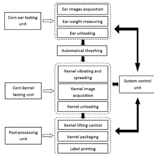
Fig.1 Principle of automatic testing system for corn
