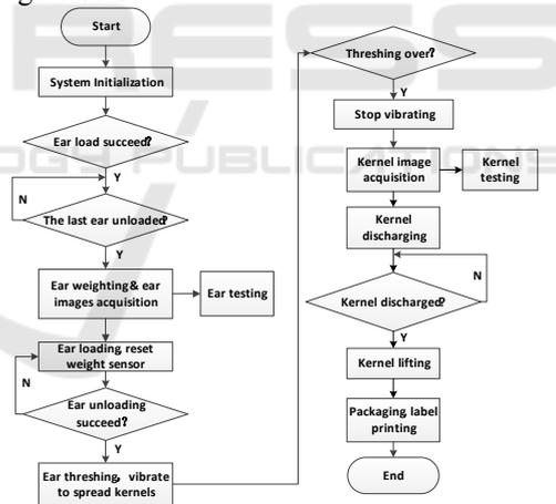
Fig.5 The flow chart of system control
