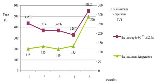
Figure 9: the comparison of the time up to 60 °C at 2.1m and the maximum temperature
