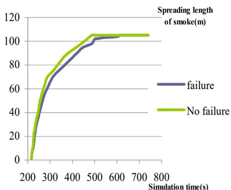
Figure 3: Comparison of smoke spreading in the central station fire with failure or no failure of sprinkler system
