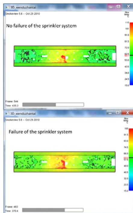
Figure 4: Station floor with a height of 2.1 m and a temperature of 60 ° C
