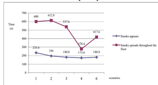
Figure 8: the time comparison of smoke appears and spreads throughout the floor
