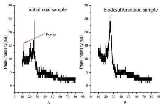
Figure 5: The XRD results of initial coal sample (A) and biodesulfurization sample (B).
