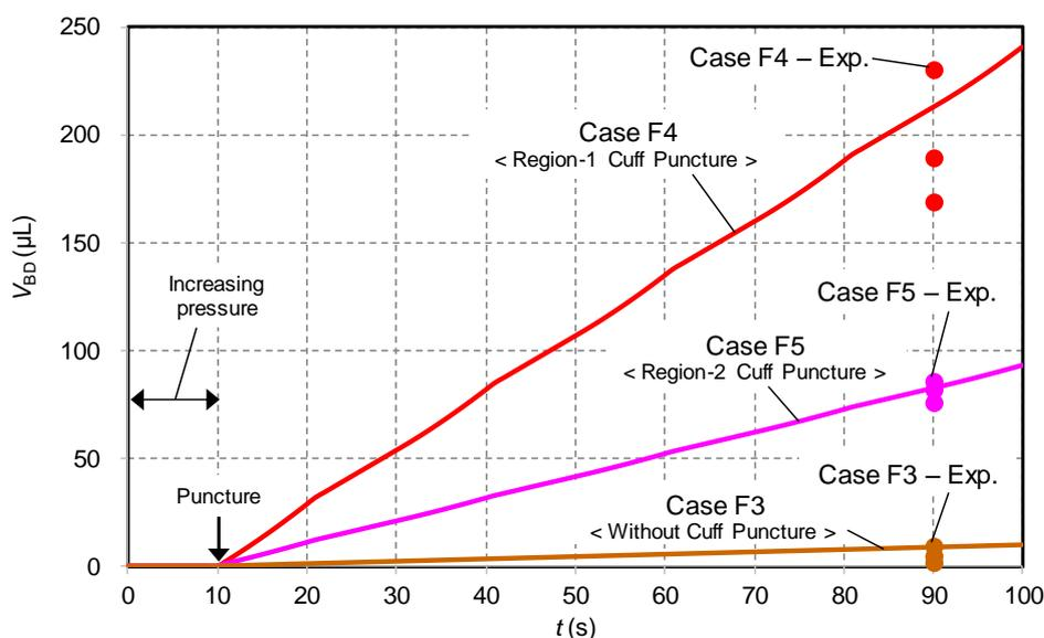
Figure 8: Comparison of the drawing blood between Hybrid Petri nets simulation.
