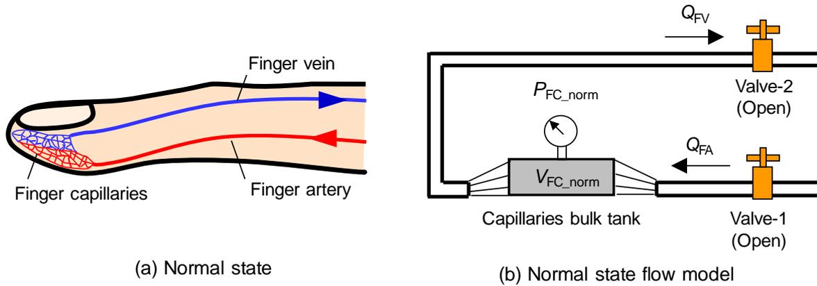
Figure 1: Close tank and pipes connection flow modelling of fingertip blood in normal state.
