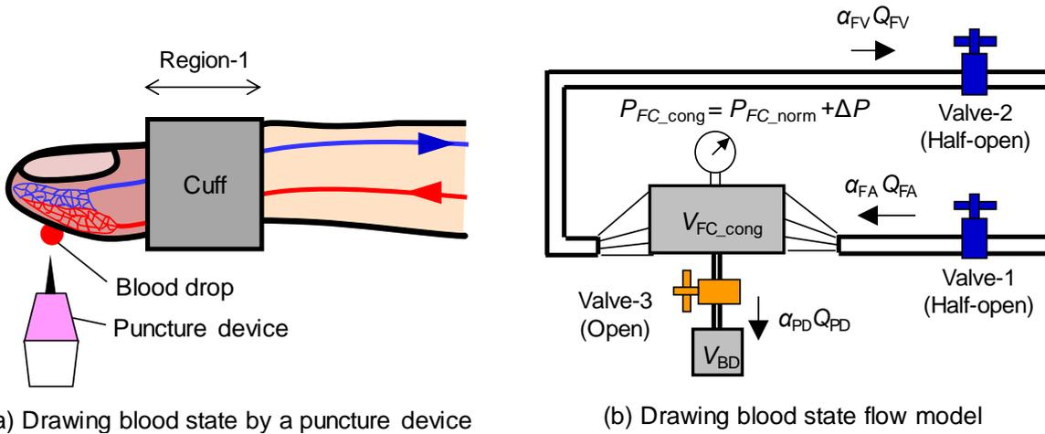
Figure 3: Close tank and pipes connection flow modelling of fingertip blood in drawing blood state with a cuff band on the region-1 by a puncture device.
