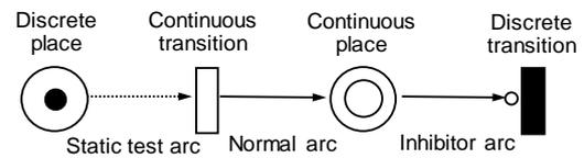
Figure 5: Basic diagram of hybrid Petri nets.
