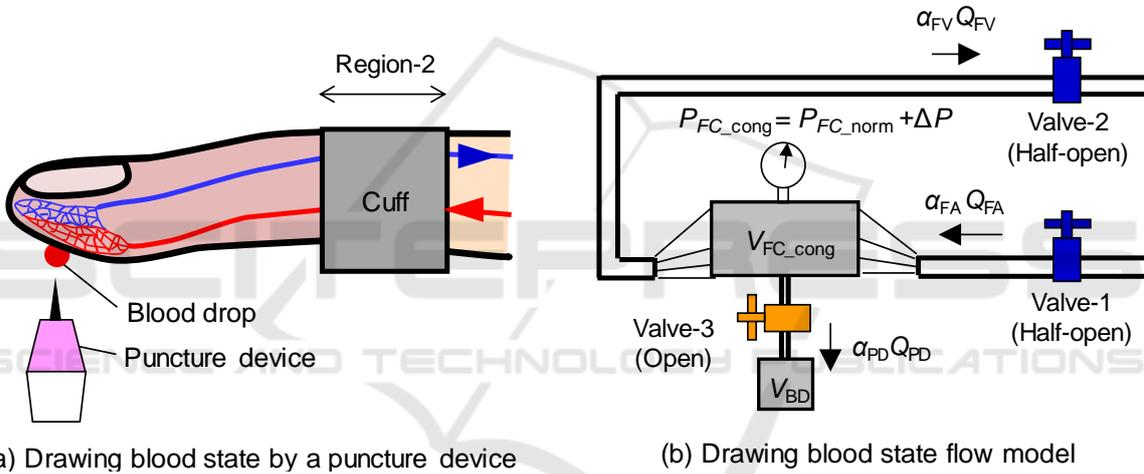
Figure 4: Close tank and pipes connection flow modelling of fingertip blood in drawing blood state with a cuff band on the region-2 by a puncture device.
