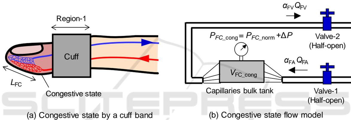
Figure 2: Close tank and pipes connection flow modelling of fingertip blood in congestive state by a cuff band.
