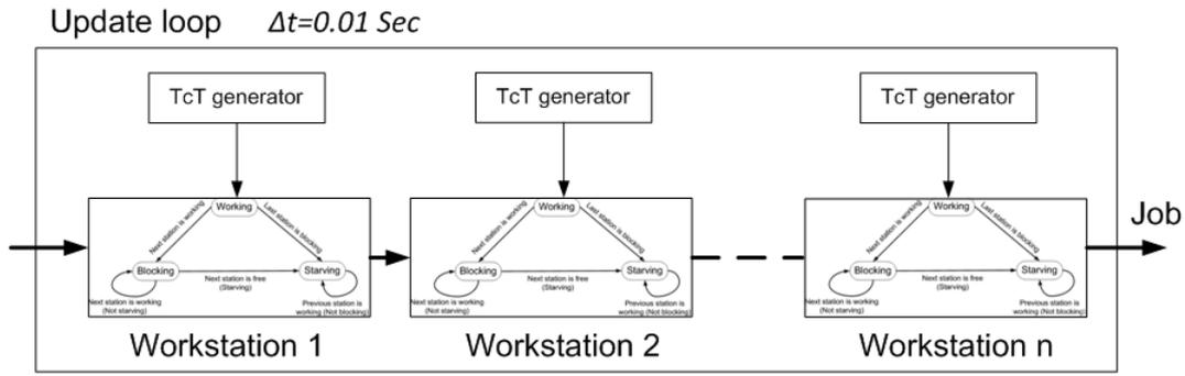
Figure 13: Welding line simulation.
