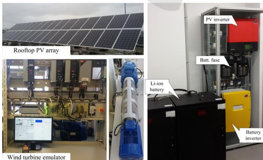
Figure 6: Illustration of the smart Residential MG acting as an EV charging station.
