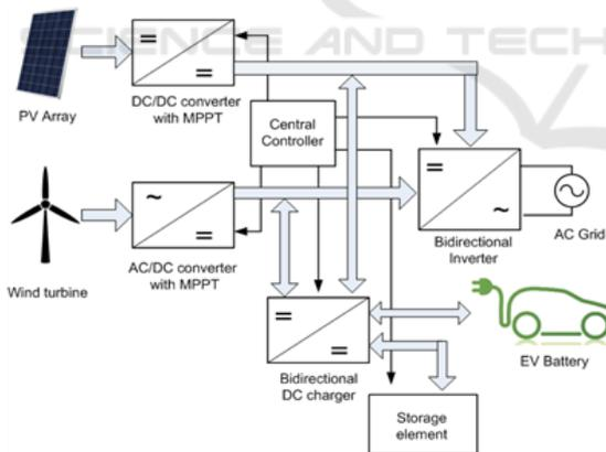
Figure 4: RES based EV charging station diagram.
