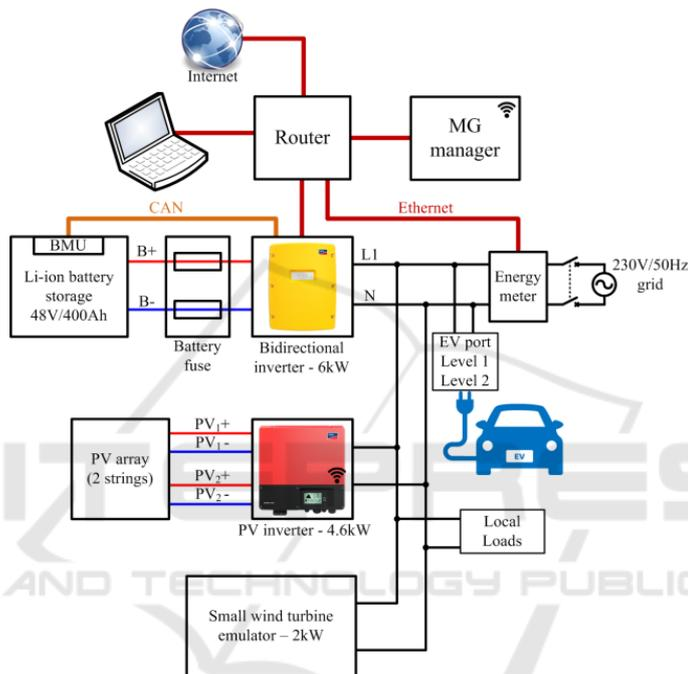
Figure 5: Diagram of the smart Residential MG designed as an EV charging station.
