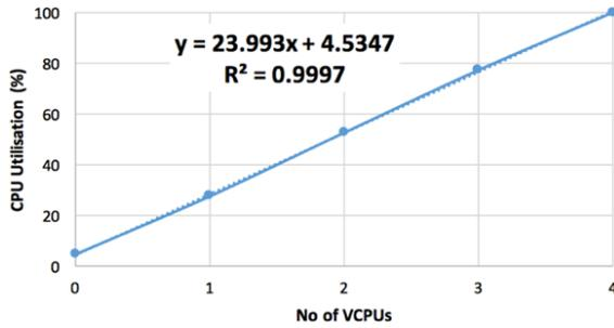
Figure 2: Number of vCPUs (VMx) vs PM CPU Utilisation (Source PMi).
