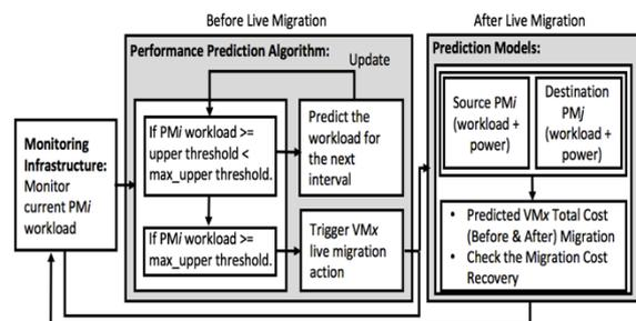
Figure 1: Performance and Energy-based Cost Prediction Framework.
