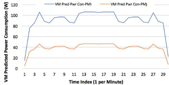
Figure 7: Predicted VMx Power Consumption on (Source PMi and Destination PMj).
