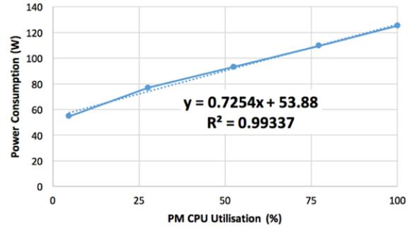
Figure 4: The PM CPU Utilisation vs Power Consumption (Source PMi).
