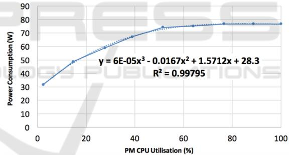
Figure 5: The PM CPU Utilisation vs Power Consumption (Destination PMj).
