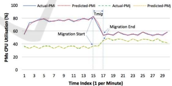
Figure 6: Predicted vs Actual in both PMs (Source  $PM_i$  and Destination  $PM_j$ ).
