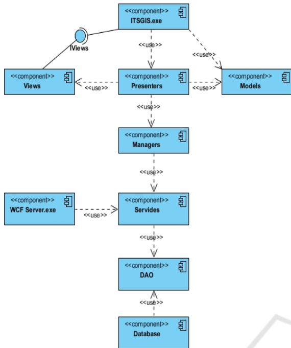
Figure 3: System components.
