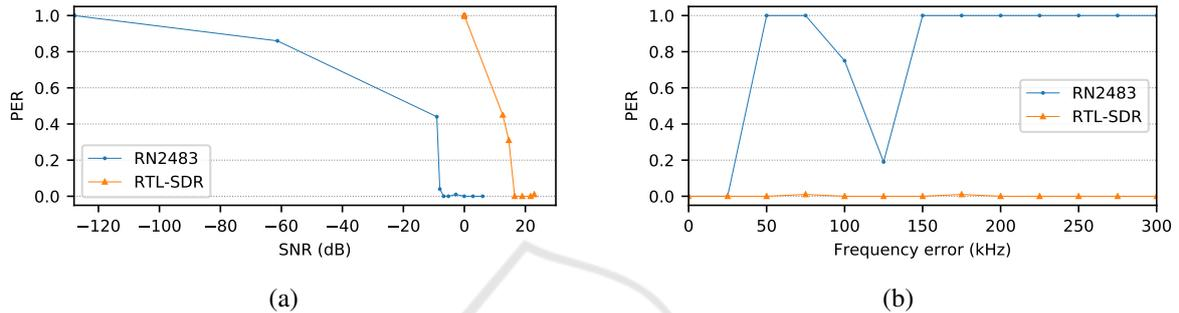
Figure 9: Comparison between the RTL-SDR using our software decoder versus a hardware RN2486 LoRa transceiver in terms of resistance to Gaussian noise (a) and resistance to frequency offset errors (b). Due to the properties of our gradient-based decoding algorithm, our decoder is shown to be unaffected by frequency errors at the cost of a significantly higher sensitivity to Gaussian noise compared to the RN2483.
