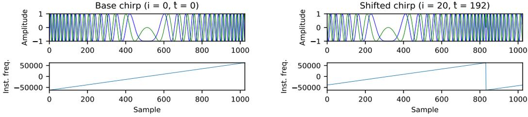
Figure 1: Example of an unmodulated LoRa base chirp and a chirp modulated with  $i = 20$ . The top row of figures shows the time domain complex signal, whereas the bottom row of figures shows the instantaneous frequencies of the signals in Hz.
