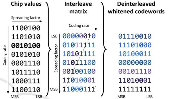
Figure 2: Diagonal deinterleaving with  $SF = 7$  and  $CR = 4$ . The bits of the third chip value are shown in bold.
