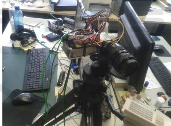
Figure 1: Test setup for recording data in a real environment. The photo shows the test setup for recording test data. The used moncamera UI-5360CP is mounted on a tripod together with a high-precision fiber gyro. During the recordings the setup was rotated around the vertical axis.
