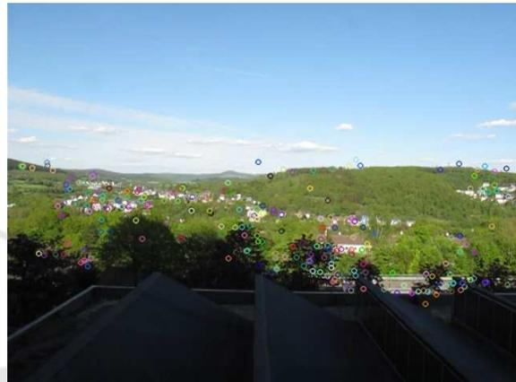
Figure 5: SIFT detector applied to a sample image. The figure illustrates the detector of the Scale Invariant Feature Transform (SIFT) algorithm. In the picture keypoints which are suitable for feature operations are drawn.
