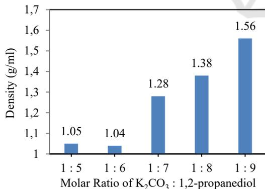
Figure 2: Molar ratio effect to DES density.
