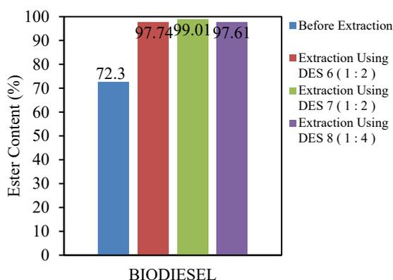
Figure 7: Comparison of biodiesel purity before and after extraction.
