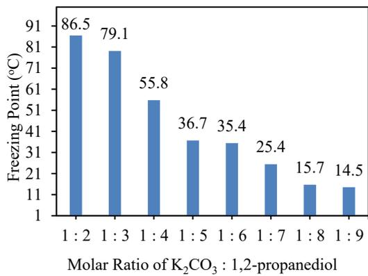
Figure 1: Molar ratio effect to DES freezing point.
