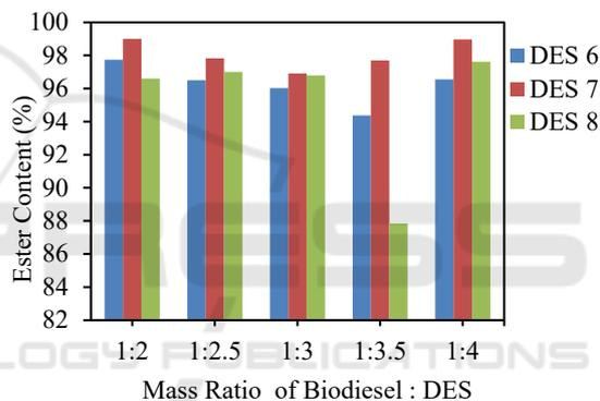
Figure 6: Ester content (%) vs. mass ratio of biodiesel: DES.
