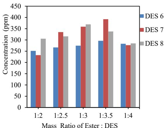
Figure 5: Concentration of extracted vitamin E vs ratio of biodiesel : DES.
