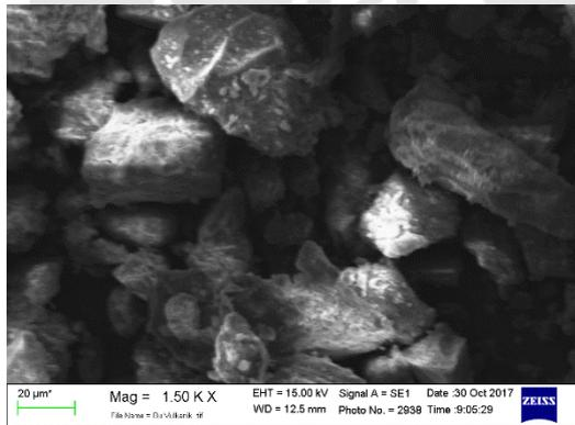
Figure 1: Magnification of Volcanic Ash Samples with SEM Test
