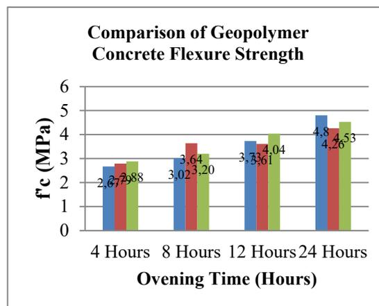
Figure 5: Flexure Strength Comparison
