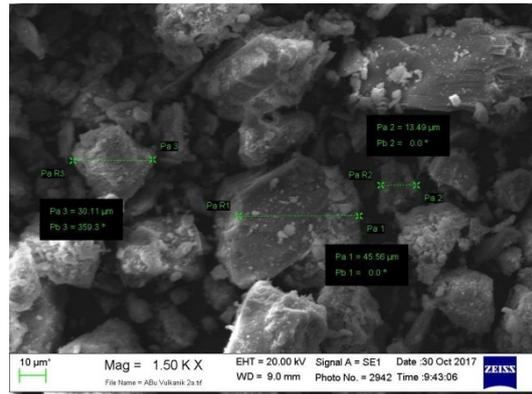
Figure 2: Magnification of Volcanic Ash Samples with SEM Test
