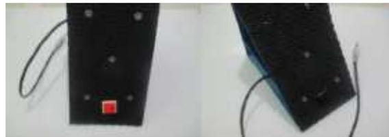
Figure 2: Box-shaped push button on foot step device on start block.
