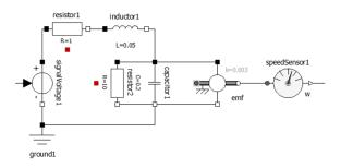
Figure 6: The DC motor, a mechanical system which rotates at a speed defined by its input voltage and measured by a speed sensor.
