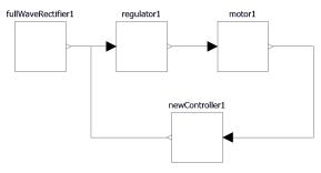
Figure 4: The box diagram of the DC motor controller, which consists of four subsystems, a full-wave rectifier, a voltage regulator, a mechanical DC motor and a PID controller.
