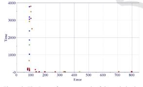
Figure 8: The Pareto front as a result of the optimization process. The points on the lower left corner corresponds to the best solutions, which minimize the time required to reach the expected regime while minimizing the error on the speed.
