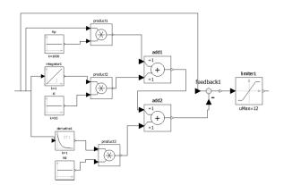
Figure 7: The PID controller, which has three coefficients which are to be optimized in order to provide the right control signals to the regulator.
