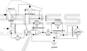
Figure 5: The regulator, which produces the voltage required to drive the DC motor based on the reference voltage provided by the rectifier and the control signal sent by the controller.
