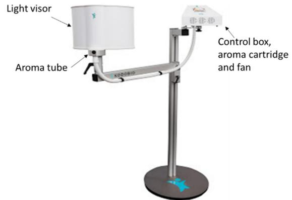
Figure 2: Light and smell delivery device.
