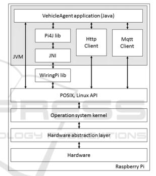
Figure 2: Raspberry Pi Architecture.
