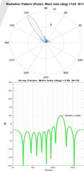
Figure 2: Array Factor plots for  $N=10$ ,  $\phi_0 = 120^\circ$ ,  $d = 0.5\lambda$ : (a) polar plot; (b) rectangular plot.
