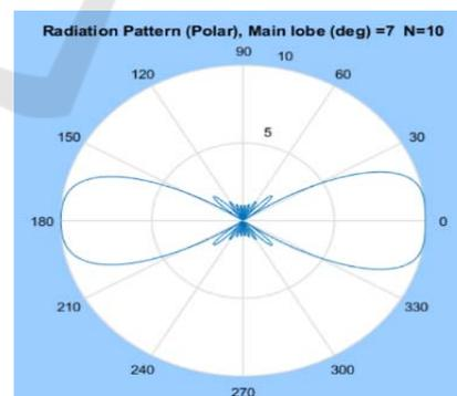
Figure 9: Array Factor Polar Plot for  $N=10$ ,  $\phi_0 = 7^{\circ}$ ,  $d = 0.5\lambda$ .
