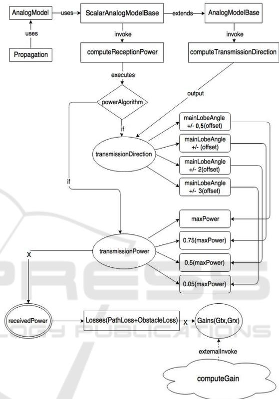
Figure 4: Logical block schema 1.
