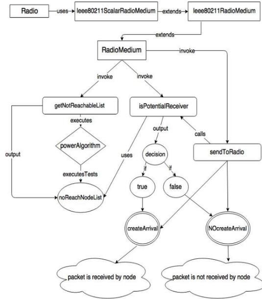
Figure 6: Logical block schema 2.
