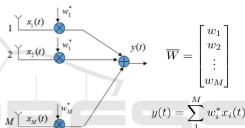
Figure 1: Smart Antenna general operation schema.
