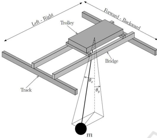
Figure 2: The typical structure of a bi-dimensional bridge crane.
