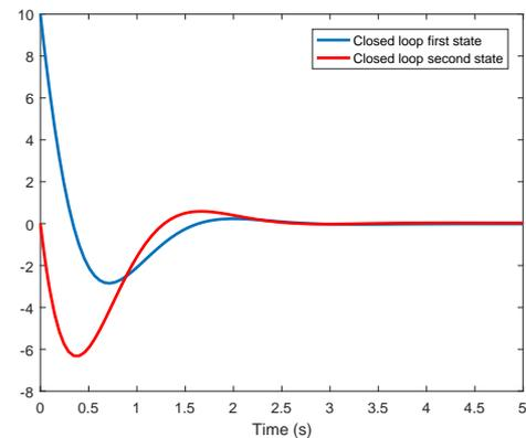
Figure 5: Bridge crane state trajectories using PID controller.
