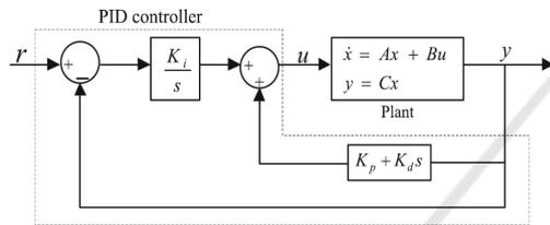
Figure 1: Feedback control structure.
