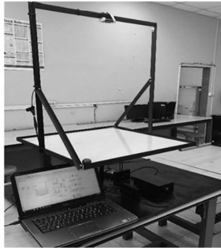
Figure 2: Experimental Ball and Plate System.
