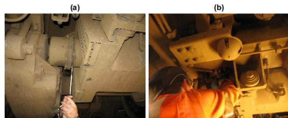
Figure 6: (a) and (b) Technician performing Class 380 curved coupler oil change.
