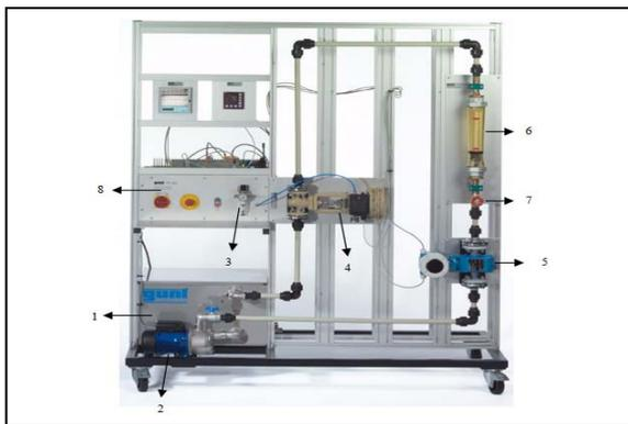
Figure 4: Experiment setup of a flow control (Abraham, 2015).
