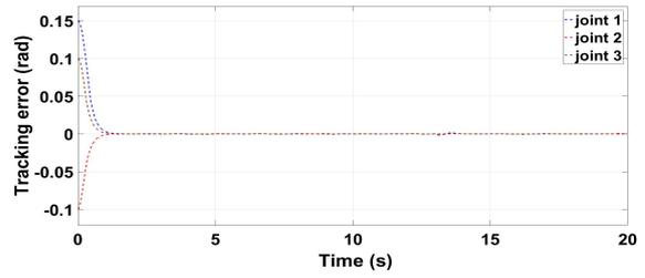
Figure 8: Joint space tracking error.
