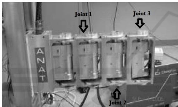
Figure 3: 3-DOF ANAT robot arm.
