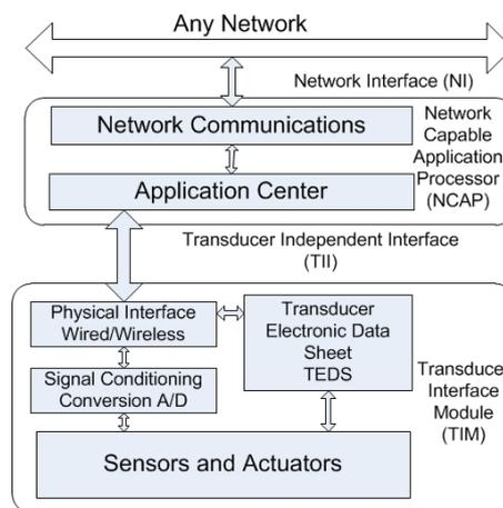
Figure 1: Structure of the smart transmitter in accordance with IEEE 1451.
