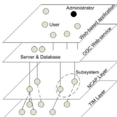
Figure 2: Structure of the smart transmitter in accordance with IEEE1451.
