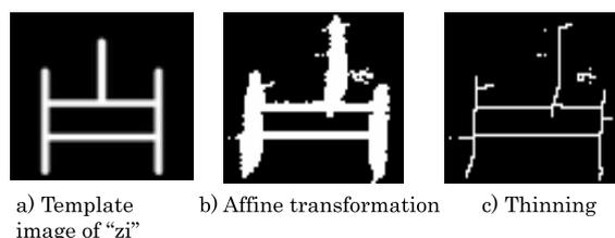
Figure 4: Feature extraction pre-processing.
