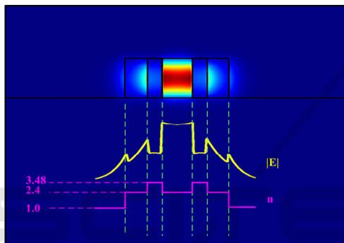
Figure 4: Electric field distribution of the multilayer waveguide.
