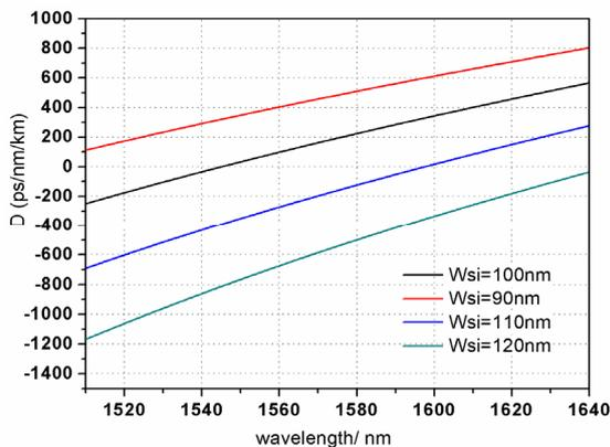
Figure 7: Waveguide dispersion curves for  $W_{Si}=90\text{nm}$ ,  $100\text{nm}$ ,  $110\text{nm}$  and  $120\text{nm}$ , respectively. The other parameters used for simulation are  $W=700\text{ nm}$ ,  $h=500\text{ nm}$ ,  $W_{\text{slot}}=200\text{ nm}$  and  $n=2.4$ .
