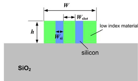
Figure 3: A schematic of the vertical multilayer hybrid silicon waveguide (in cross view).
