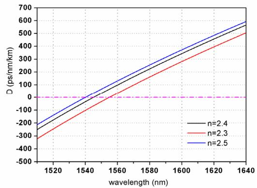
Figure 5: Waveguide dispersion curves for  $n=2.3, 2.4$  and  $2.5$ , respectively. The other parameters are  $W=700\text{ nm}$ ,  $h=500\text{ nm}$ ,  $W_{\text{Si}}=100\text{ nm}$  and  $W_{\text{slot}}=200\text{ nm}$ .
