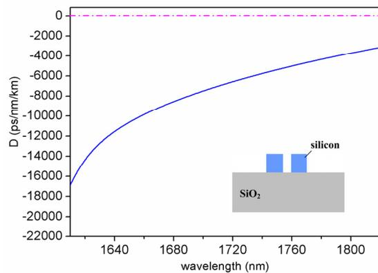
Figure 2: Simulated dispersion curve of a silicon vertical slot waveguide. The top silicon layer thickness is 340nm. The widths of the slot and silicon rail are 100nm and 200nm, respectively.
