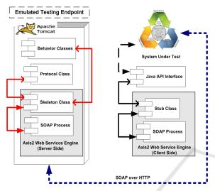
Figure 4: Testing runtime environment deployment view.
