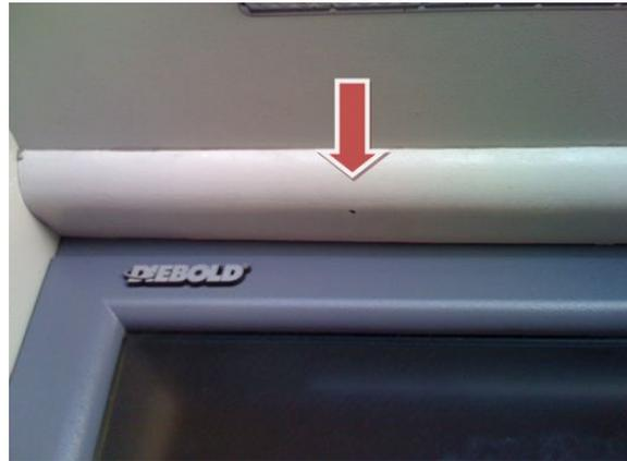
Figure 1: A micro camera in a cash machine case. Source: <http://krebsonsecurity.com/>.
