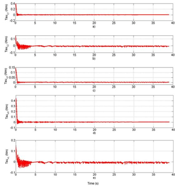
Figure 6: (a) The input torque of the joint 1, (b) The input torque of the joint 2 (c) The input torque of the joint 3, (d) The input torque of the right wheel 1, (e) The input torque of the left wheel.
