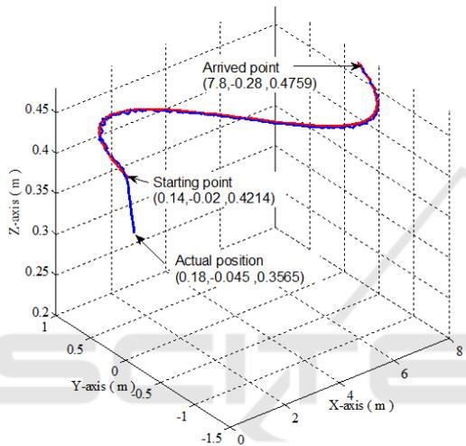
Figure 4: Desired trajectory of manipulator's end effector.
