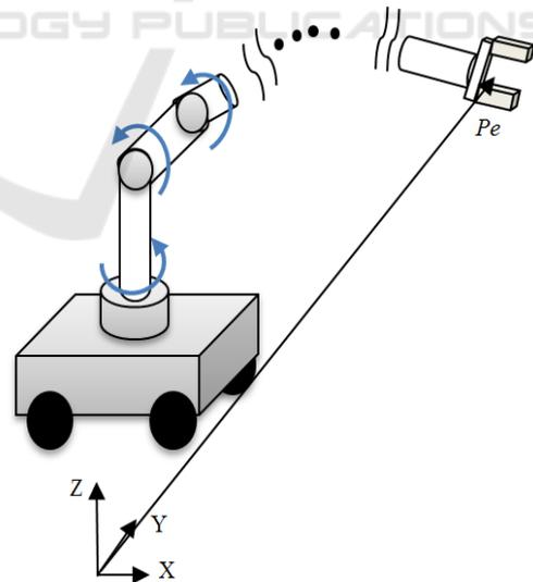
Figure 1:  $n$ -DOF mobile manipulator robot.
