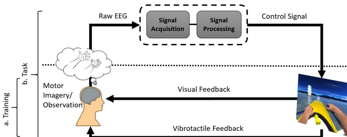
Figure 2: Neurofeedback loop. (a) During the training session, the user is performing in a randomized order MI combined with motor observation of the virtual hands rowing while vibrotactile feedback is delivered to the corresponding hand. (b) The user relies on MI alone in order to control the virtual hands in a closed-loop system after training.
