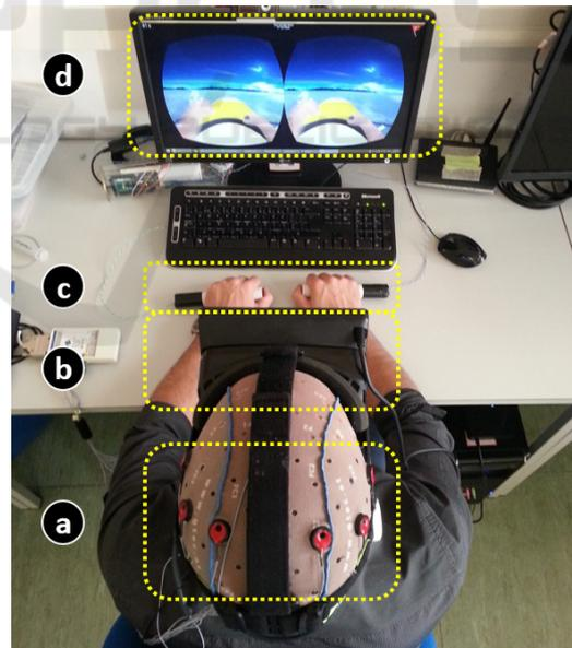
Figure 1: Experimental setup (a) EEG cap with 8 active electrodes, (b) HMD, (c) vibrotactile modules, (d) BCI feedback.
