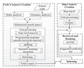
Figure 1: Functional block diagram of MBuM.
