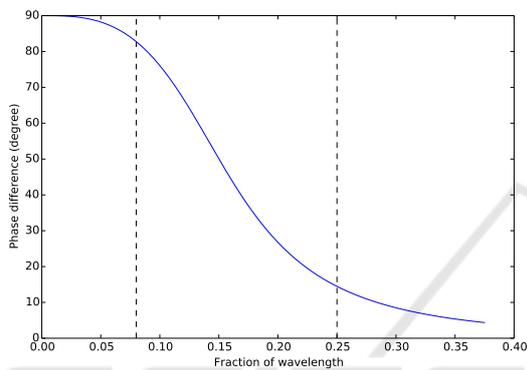
Figure 3: Plot showing the difference in phase as a result of distance from the transmitter. The interval between the vertical lines indicates the best area of operation.
