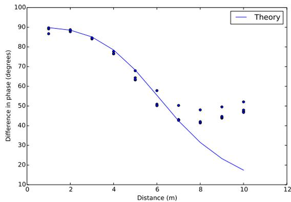
Figure 9: Theoretical and measured phase difference between magnetic and electric component of a 7.03 MHz signal in the near-field.
