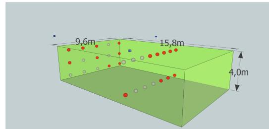
Figure 4: The placement of sensor nodes and base stations during the experiment. The spheres are sensors and the boxes are base stations.
