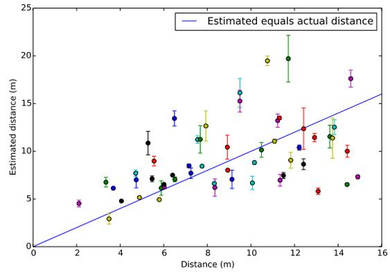
Figure 7: The estimated distance between the individual nodes and the base stations compared to the actual distance.
