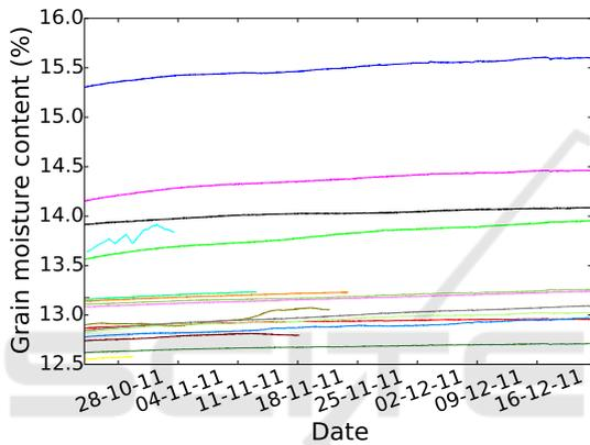
Figure 6: The moisture content wet-basis of the grain. Calculated using the modified Henderson equation (ASAE Standards, 1999).
