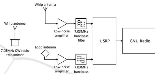
Figure 8: Diagram of the experimental setup.
