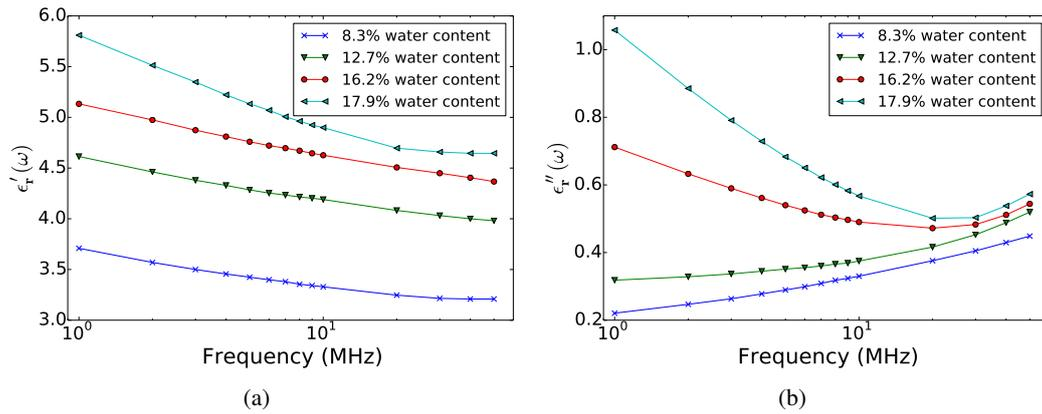
Figure 2: The permittivity of 'Nebred' hard red wheat at  $24^{\circ}\text{C}$  and the indicated moisture content. The density of the wheat was  $768 \text{ kg/m}^3$  at 13% moisture content. (a) shows the relative permittivity over a range of moisture content, and (b) shows the loss factor. Graph recreated from (Nelson, 1965).
