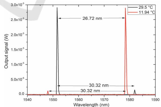
Figure 4: Generated CW laser lines at both wavelength tuning limits.
