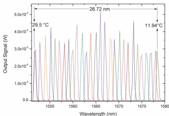
Figure 3: Measured CW laser line wavelength spectra tuned by Hi-Bi FOLM fiber loop temperature variations.
