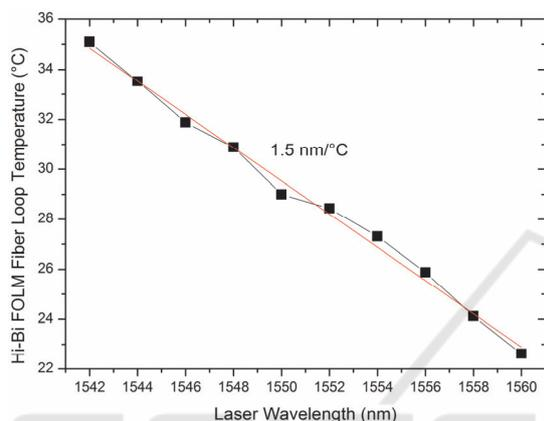
Figure 5: Actively Q-switched laser line wavelength tuning on Hi-Bi FOLM fiber loop temperature variations.
