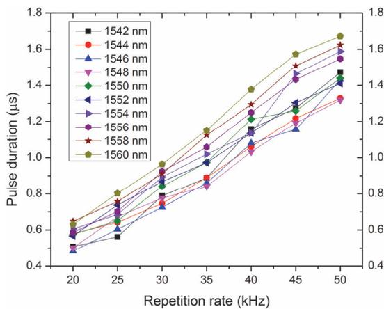
Figure 8: Pulse duration on repetition rate variations of different wavelength tunings for actively Q-switched laser operation.
