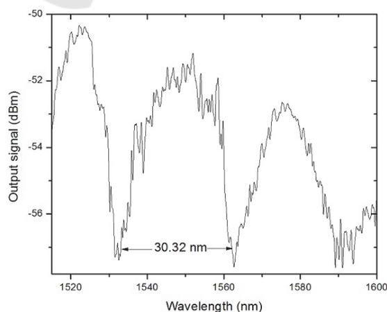
Figure 2: Hi-Bi FOLM measured transmission spectrum.
