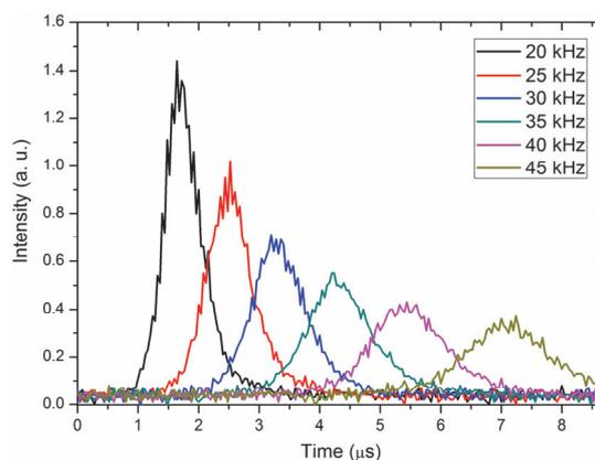
Figure 6: Actively Q-switched pulses profile on repetition rate variations for generated laser wavelength at room temperature.
