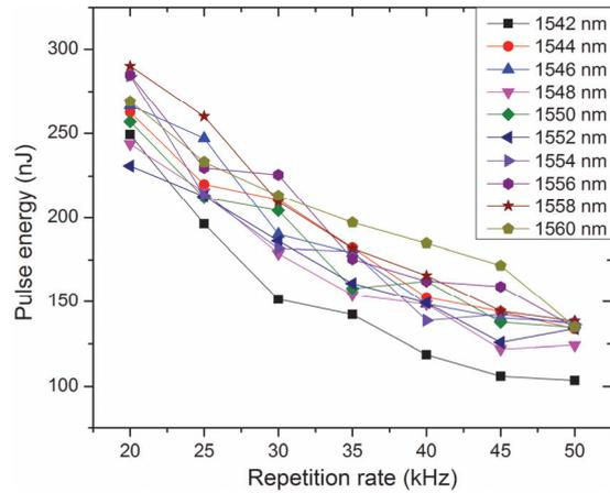
Figure 9: Pulse energy on repetition rate variations of different wavelength tunings for actively Q-switched laser operation.
