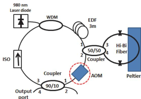
Figure 1: Proposed ring cavity Erbium-doped fiber laser experimental setup.
