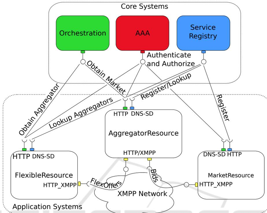
Fig. 7. Software architecture of the Virtual Market of Energy.
