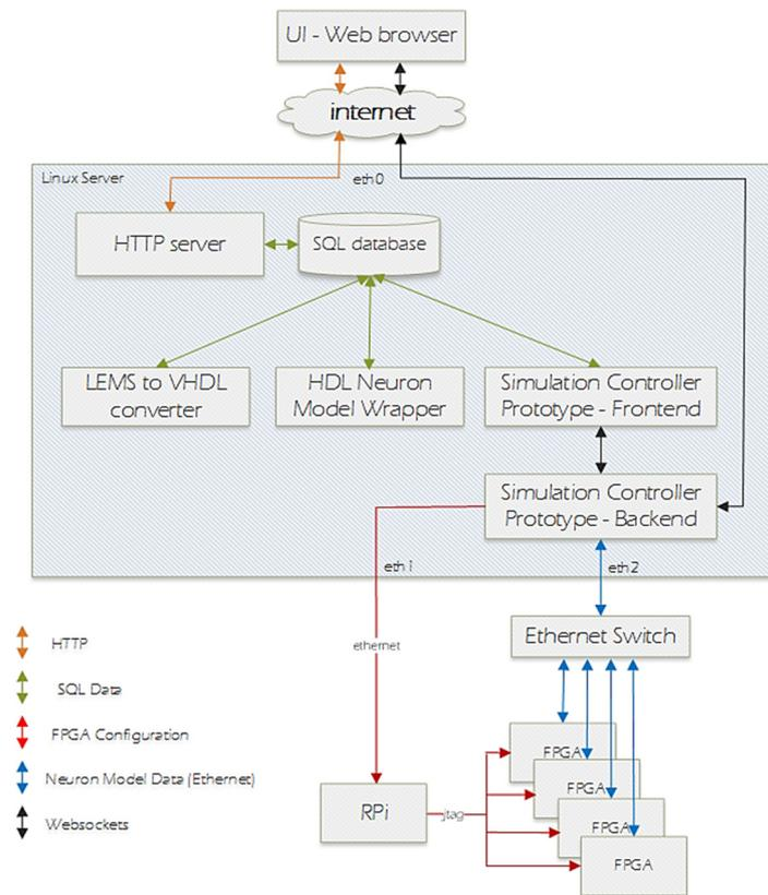
Figure 1: Prototype System Architecture.
