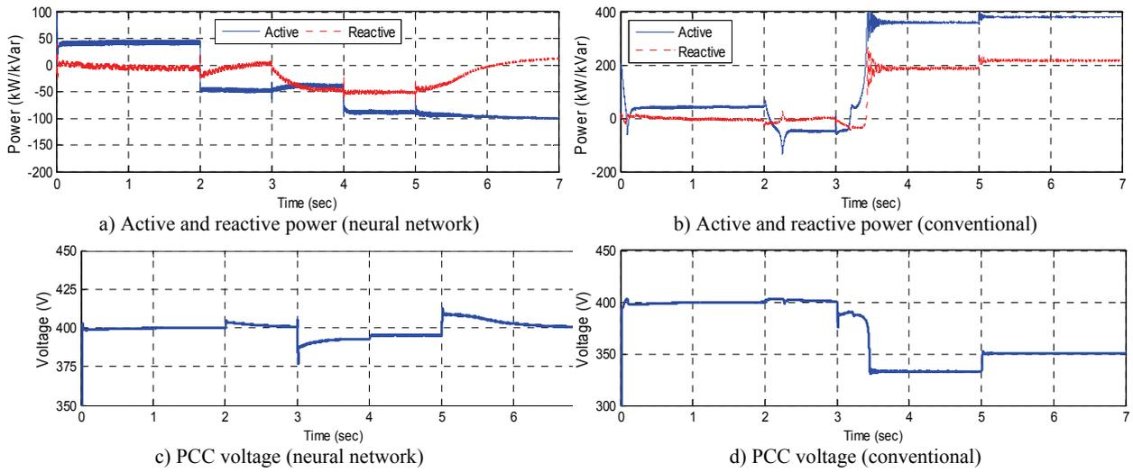
Figure 4: PV-inverter with constraints using conventional and neural network controllers.
