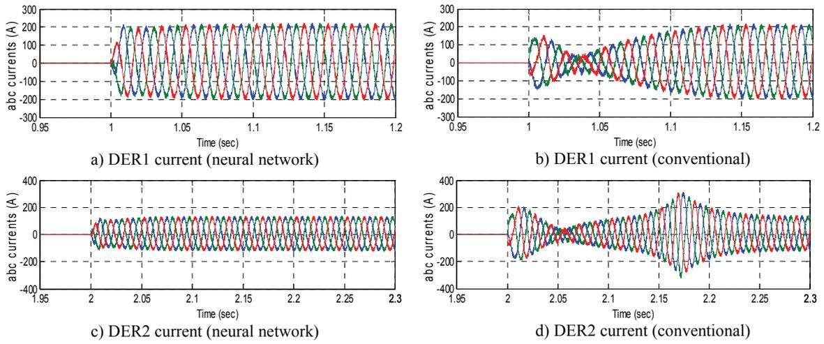
Figure 6: Three-phase currents when connecting DERs to the grid without synchronization control.
