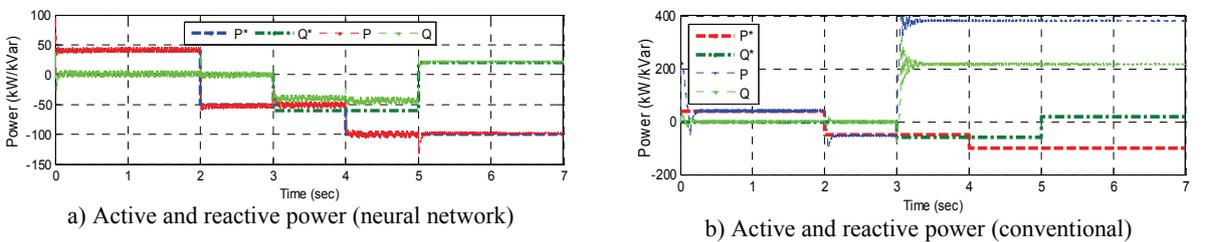
Figure 3: PQ-inverter DER with constraints using conventional and neural network controllers.
