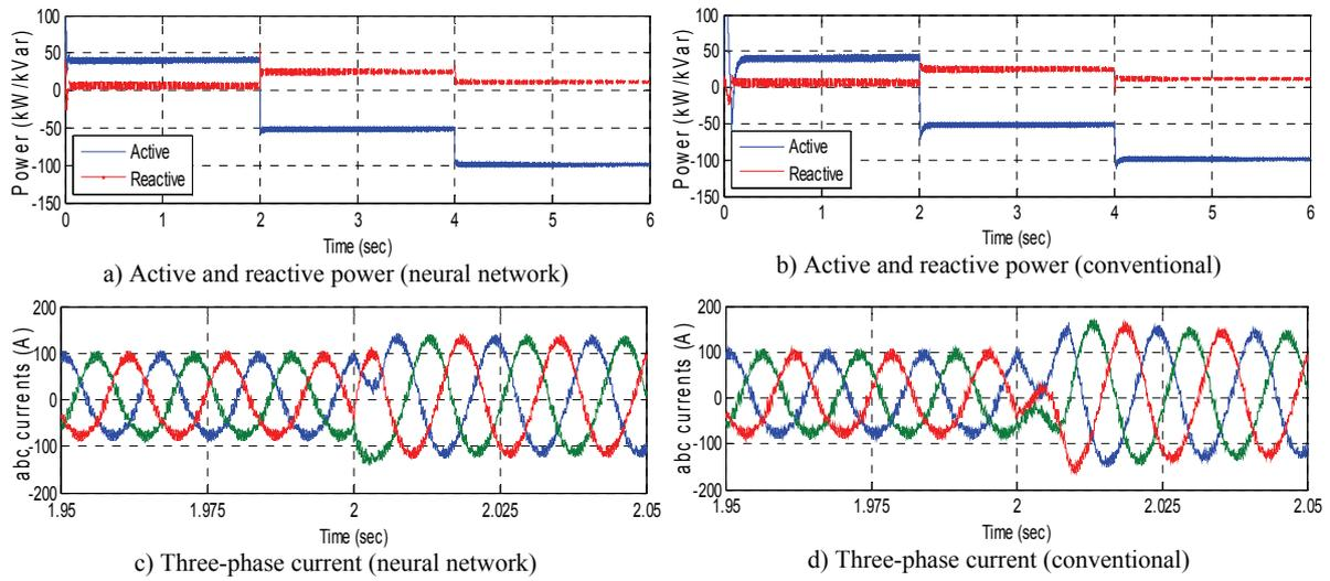
Figure 1: Performance of PQ-inverter DER using conventional and neural network controllers ( $T_s=1ms$ ).
