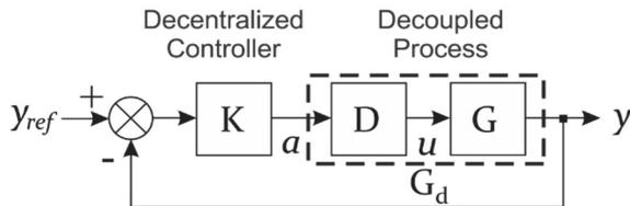
Figure 4: Decentralized controller with compensator.
