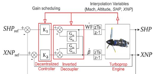
Figure 12: Control laws implemented with an incremental algorithm.
