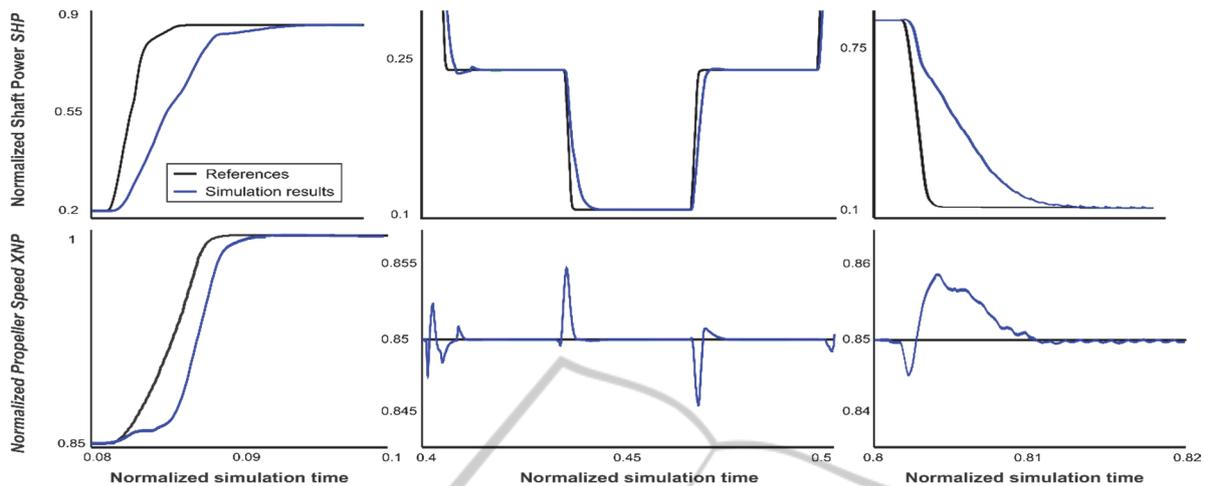
Figure 14: Simulation results (zoom on some transient states).
