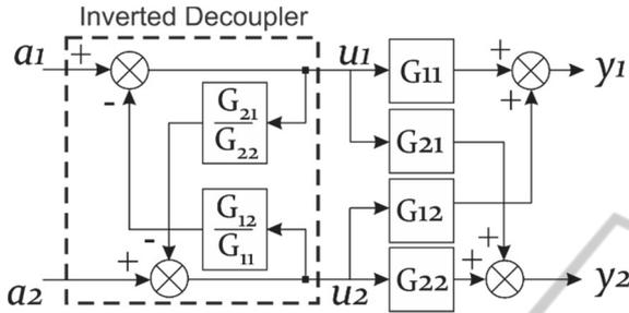
Figure 5: Scheme of the inverted decoupler.
