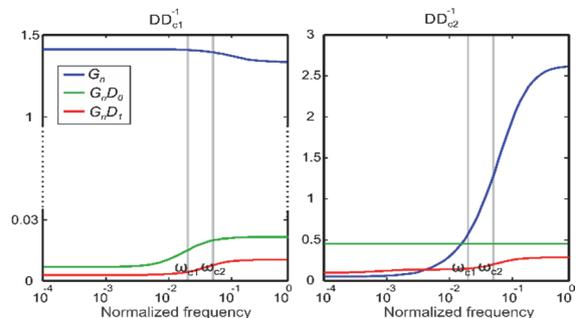
Figure 7:  $DD^{-1}$  of the process and decoupled processes.
