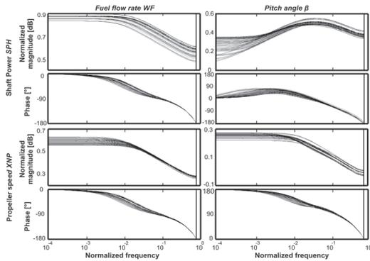
Figure 1: Bode diagrams of the identified models.
