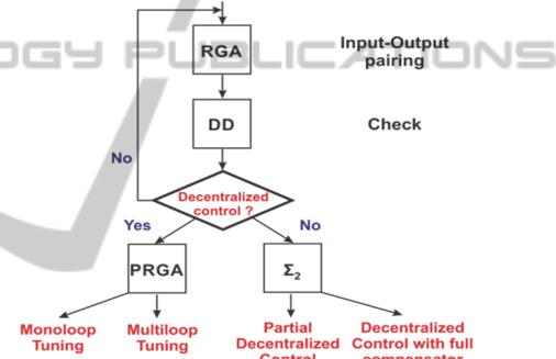
Figure 2: Procedure of interaction analysis.
