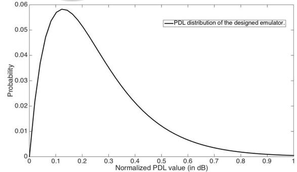
Figure 2: The statistical result of the designed emulator obeys Maxwellian distribution.
