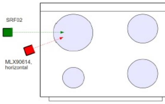
Figure 4: Positioning on workspace (20 cm to the left side of burner) of SRF02 sensor for detecting presence of utensil on burner and MLX90614 sensor for measuring utensil temperature.
