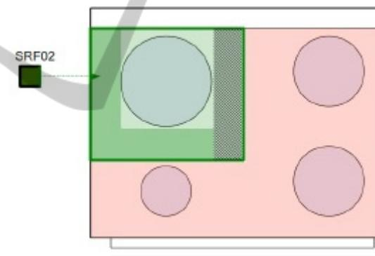
Figure 17: The actual situation: the inner rectangle (light green zone) represents the real "on-burner" zone. A utensil inside this zone is detected by SRF02. The outer rectangle (dark green) zone represents the false positive zone of SRF02 sensor where a utensil is detected as "on-burner" and in reality it is outside burner. The shaded zone represents the dead zone of the sensor.
