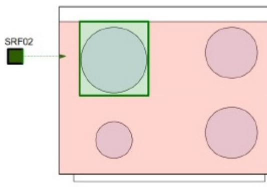
Figure 16: The ideal situation: if utensil is located inside the rectangle (green zone), then it is on burner, otherwise (pink zone) it is not.
