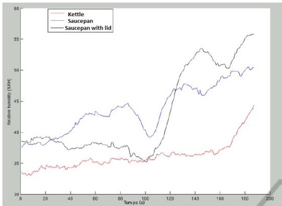
Figure 18: Relative humidity when water boils in: kettle, saucepan, and saucepan with lid.
