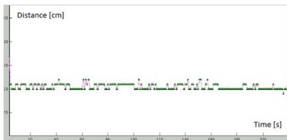
Figure 14: Distance measurements [cm] by SRF02 sensor while cooking meat in a frying pan placed in the middle of burner.
