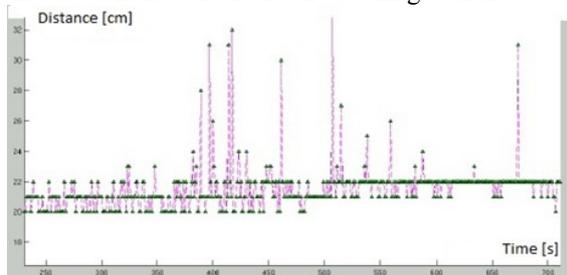
Figure 15: Distance measurements [cm] by SRF02 sensor while heating water in a saucepan placed in the middle of burner.
