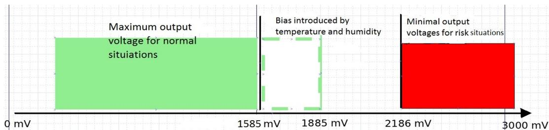
Figure 7: Output voltages of Alcohol (TGS2620) and VOC (MICS5521) sensors in normal and risk situations.
