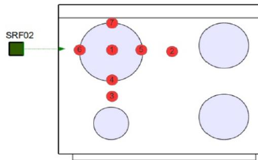
Figure 13: Positions of the center of utensil on burner for testing SRF02 sensor.
