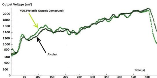
Figure 10: Output voltages of MICS5521 VOC and TGS2620 Alcohol sensors when frying oil during 8 minutes.
