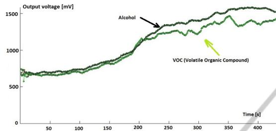
Figure 8: Output voltages of MICS5521 VOC and TGS2620 Alcohol sensors when cooking hotdogs in a frying pan.
