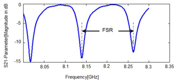
Figure 4: Transmission parameter of the PMMA structure in the simulation.
