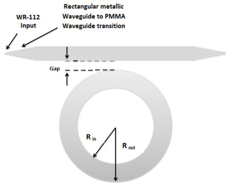
Figure 2: The top view of waveguide and ring resonator structure.
