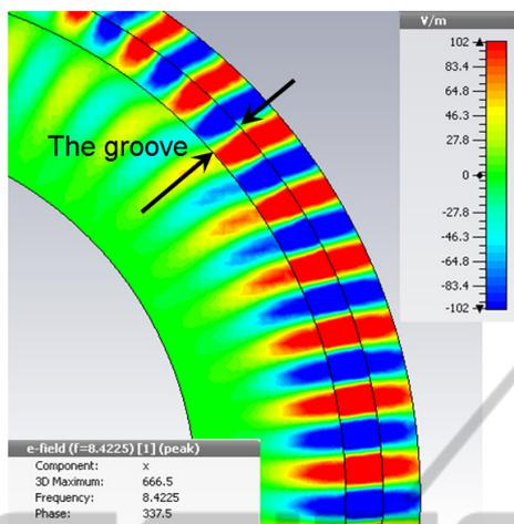
Figure 7: simulated 3D electric field (x component) distribution of the ring resonator with a groove on the surface. The electromagnetic waves break when they meet the groove.
