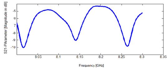
Figure 6: The plotted transmission Parameter of the ring resonator structure in the implementation.
