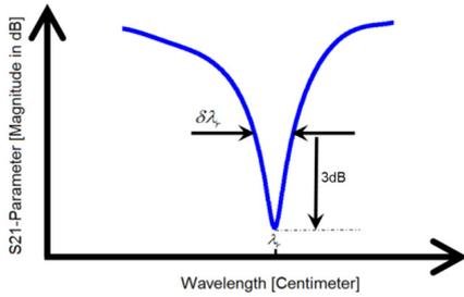
Figure 1: Exhibition of the linewidth in a resonance frequency for calculating the quality factor. .
