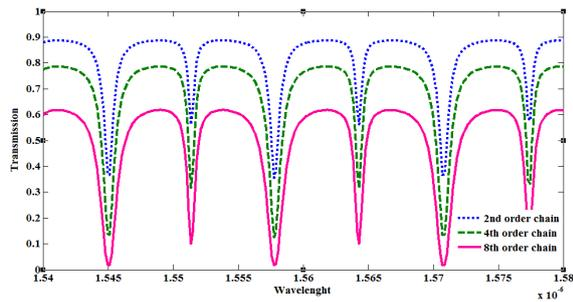
Figure 6: Various orders of single-channel SCISSOR filter imposed by Thue-Morse sequence ( $n_{\text{waveguide}}=1.5$ ,  $n_{\text{ring}}=3$ ,  $c=0.8$ ,  $l_a=20\mu\text{m}$ ,  $\alpha=50(\mu\text{m})^{-1}$ ,  $r_a=10\mu\text{m}$ ,  $r_b=r_a$ ,  $\gamma=0.1$ ).
