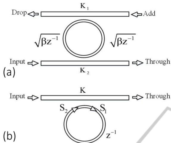
Figure 3: Schematic of the unit cells. (a) A ring resonator with two directional couplers  $K_1$  and  $K_2$ .  $\sqrt{\beta z^{-1}}$  is the amplitude transmission of the signal.
