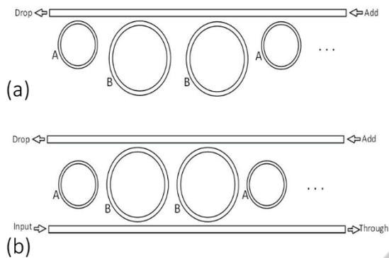
Figure 1: One dimensional micro-ring resonator chains. (a) Single channel SCISSOR chain whose system response implement multiple poles, (b) Double channel SCISSOR with separate resonances.
