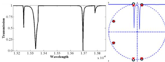
Figure 4: Fourth order double-channel SCISSOR filter with coupling coefficient 0.4, the radius  $r_a = 20 \mu\text{m}$  and  $r_b = 2r_a$ .
