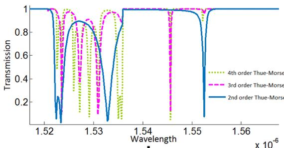
Figure 5: Design of double-channel SCISSOR filters for various class factors of Thue-Morse chains. The power coupling factor is 0.4 at both couplers,  $r_a = 20 \mu\text{m}$ ,  $r_b = 2r_a$ , refractive index is equal to 1.44, and rings are separated by the straight waveguide with the length of  $r_a$  and the effect of loss is neglected.
