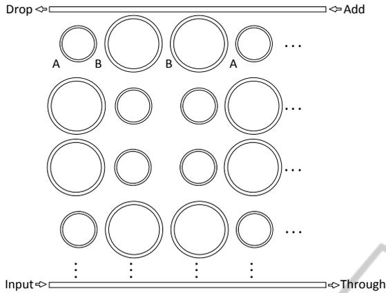
Figure 2: Two dimensional micro-ring resonator structure implementing multiple poles.
