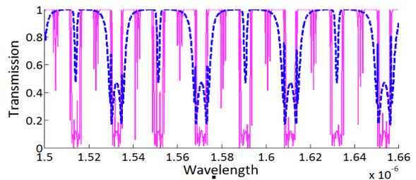
Figure 9: Transmission spectra for the first [blue] and second [pink] order Thue-Morse imposed dual-ring double-channel SCISSOR structure.
