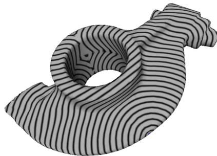
Figure 1: Geodesic distance radius from a starting point on genus 1 rocket arm model. At the hole (tunnel), we can see some sharp pattern which can be recognize as geodesic path came from different directions.
