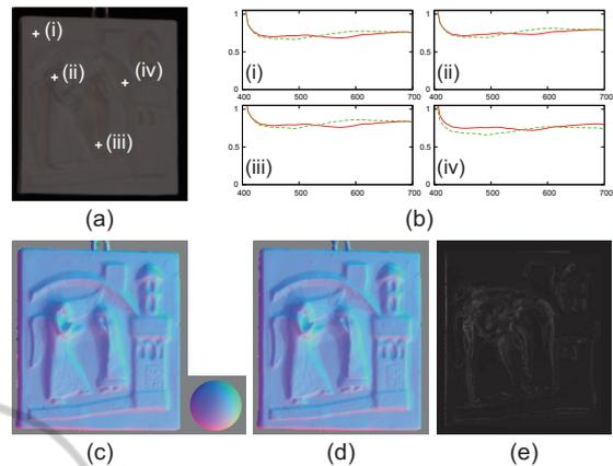
Figure 2: The estimated spectral reflectances (b) at four points on the plaster relief (a). The red-lines stand for the straightforward method using 120 images and the green-dotted lines stand for our proposed method using 9 images. (c), (d), and (e) show the normals estimated by using the straightforward method and our method and their difference respectively. Those results demonstrates that our method performs as well as the straightforward method.
