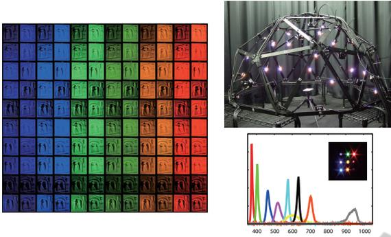
Figure 1: The images of a plaster relief (left) captured by using the multispectral light stage (right). The pixel values are scaled for display purpose.
