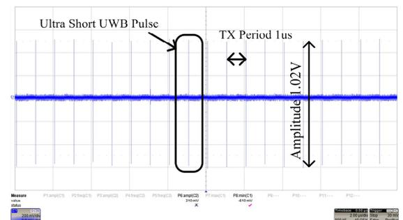
Figure 9: UWB pulses @ 1 Mbps pulse rate.
