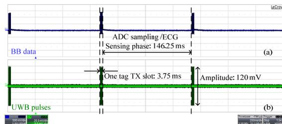
Figure 7: UWB TX interleaving with ADC sampling.
