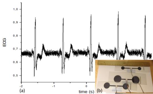
Figure 10: Measured ECG by inkjet-printed electrodes.
