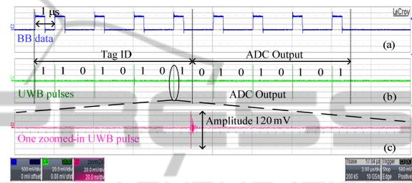
Figure 8: UWB TX of 1 ADC data @ 1 Mbps pulse rate.
