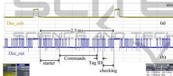
Figure 6: UHF-RFID command RX.
