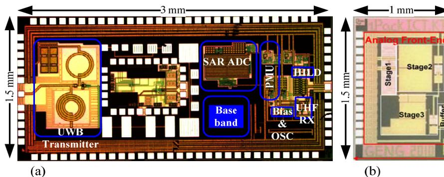
Figure 5: Silicon die photos of UWB-RFID tag (a) with ECG sensing (b).
