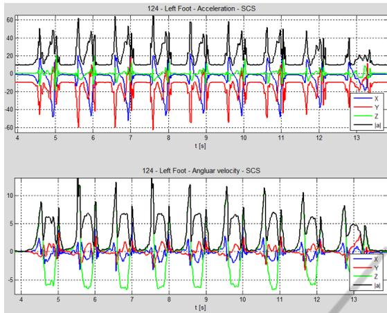
Figure 2: Acquired acceleration and angular velocity with respect to SCS (black – length of the vector).
