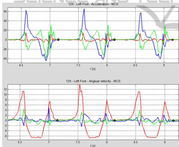
Figure 4: Acceleration and angular velocity with respect to MCS (black–begin of integration).
