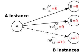
Figure 2: An example of value assignment for variables modelling the references. The instance of class  $A$  references three instances of class  $B$ . The dashed line indicates that this variable is optional why its domain includes  $\text{jokers}$ .
