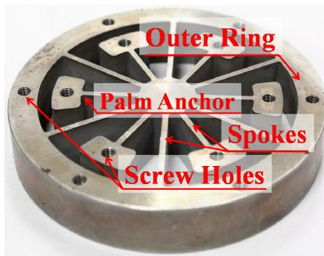
Figure 4: Photograph of Orange-slice-alike flexible body.
